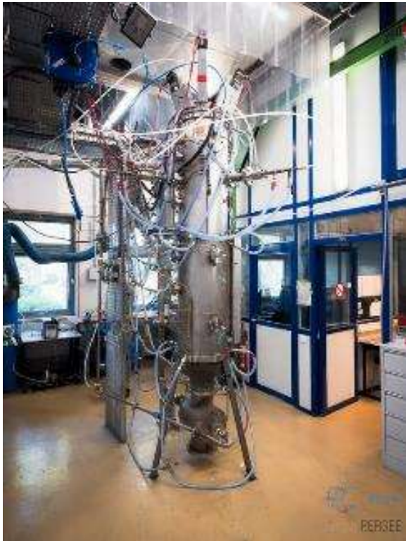
Figure 22 - Torche plasma du centre Persée - Mines ParisTech - Sophia Antipolis
