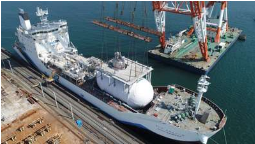
Figure 14 – World's first liquefied hydrogen carrier launched in Japan. Ce navire de 120m transportera 90t d'hydrogène
